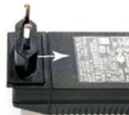
Image 2-18 Mounting the plug
