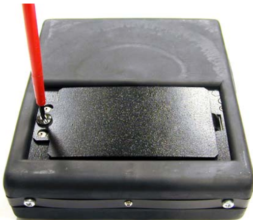
Image 2-13 Open the battery cover
